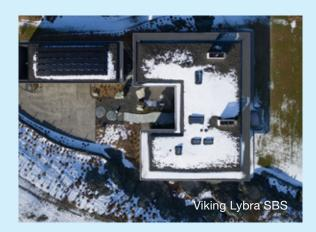
SBS membranes have a lower melt point and high cold-flexibility credentials allowing them to be exposed to lower temperatures without fracturing. The SBS system stocked in New Zealand and marketed exclusively by Viking Roofspec is called 'Viking Lybra SBS'.
