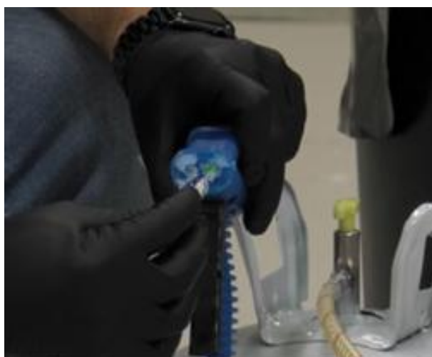
Application of petroleum jelly to spray gun
