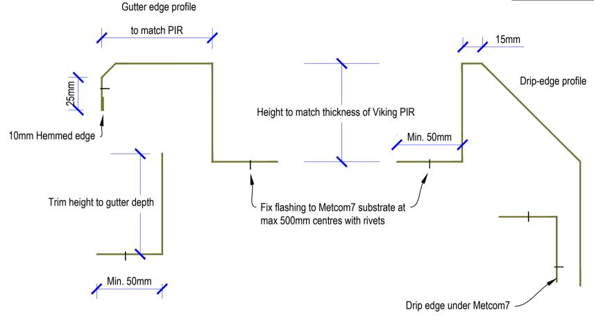
NOTE: These are indications for flashings only. Not supplied by Viking Roofspec. Flashing 55g metal riveted to Metcom7 substrate and to other flashings at 500mm max centres Metcom7 profile is 36mm deep
