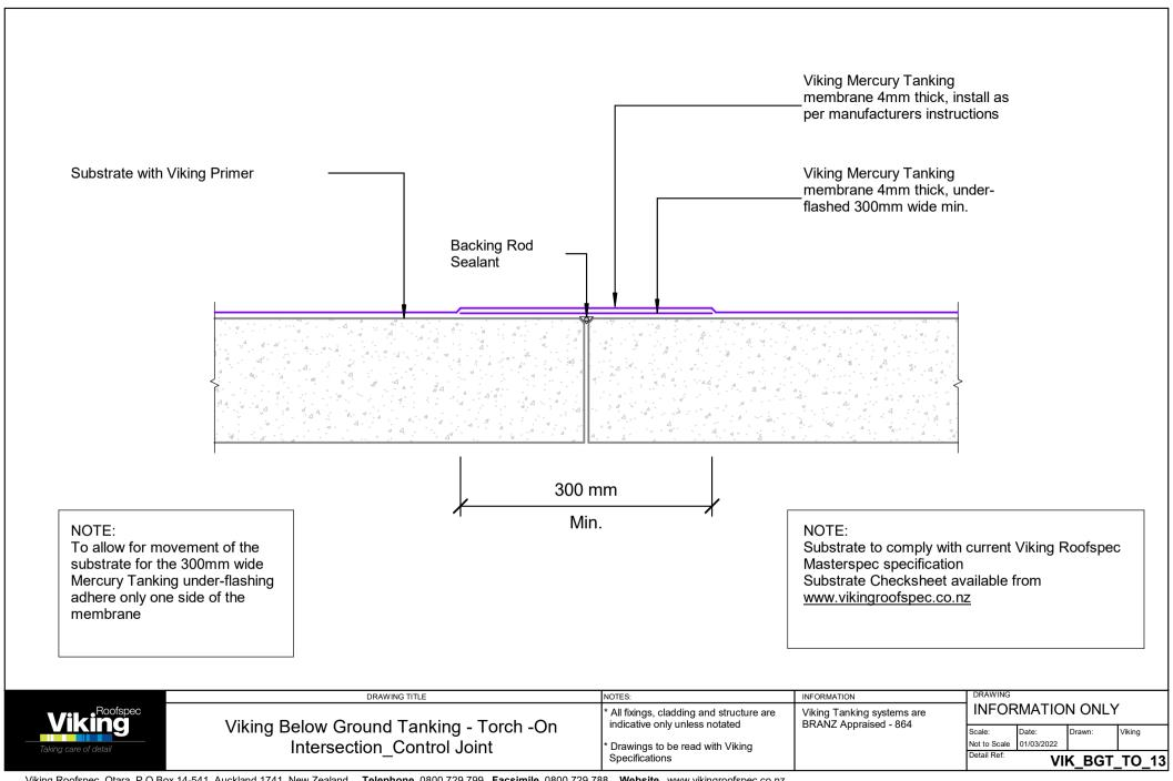
Substrate to comply with current Viking Roofspec Masterspec specification
