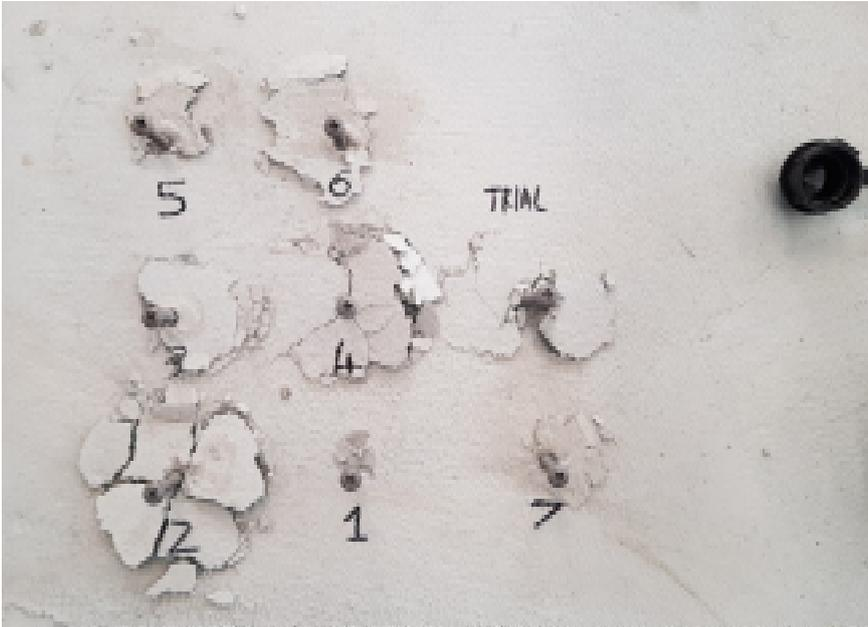
Figure 5-6. Carlisle HD14-10 fasteners after loading in concrete
