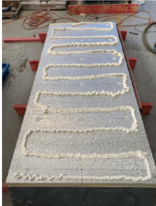
Figure 9-9. Viking Soudafoam applied to PIR panel
