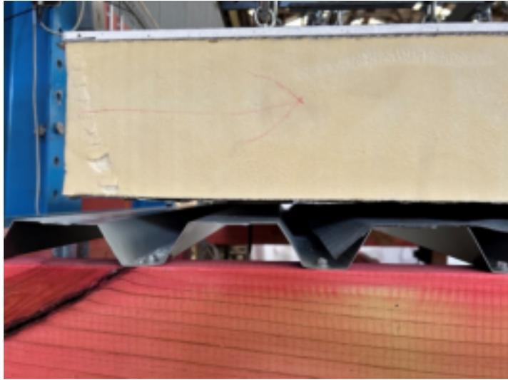
Figure 9-19. Washer pulling through PIR affixed to ST900
