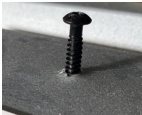
Figure 5-3. Carlisle HP-X fastener showing upturned lip
