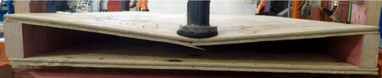
Figure 8-11. Rupture under ULS load (Location 3, Sample 3)
