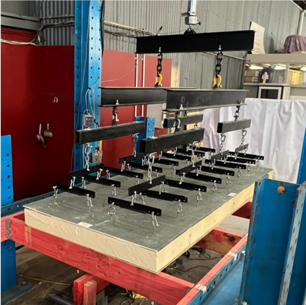
Figure 9-1. Whiffle tree attached to specimen
