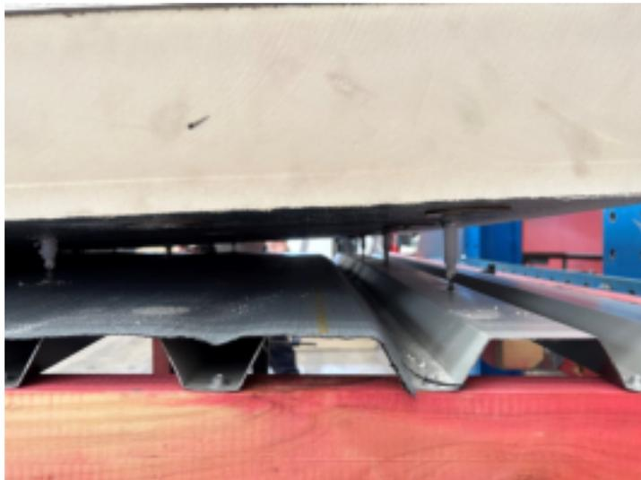
Figure 9-20. Washer pulling through PIR (during post-test removal)
