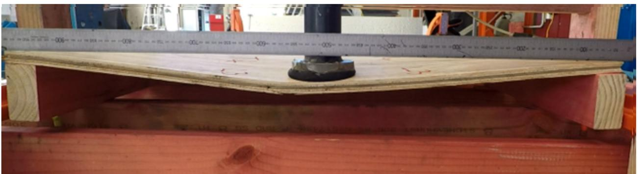
Figure 8-10. Deflection under ULS load (Location 3, Sample 2)
