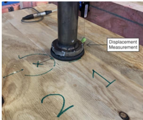
Figure 8-6. Example of point load application and measurement
