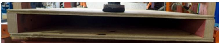
Figure 8-8. SLS residual deflection (Location 3, Sample 3)
